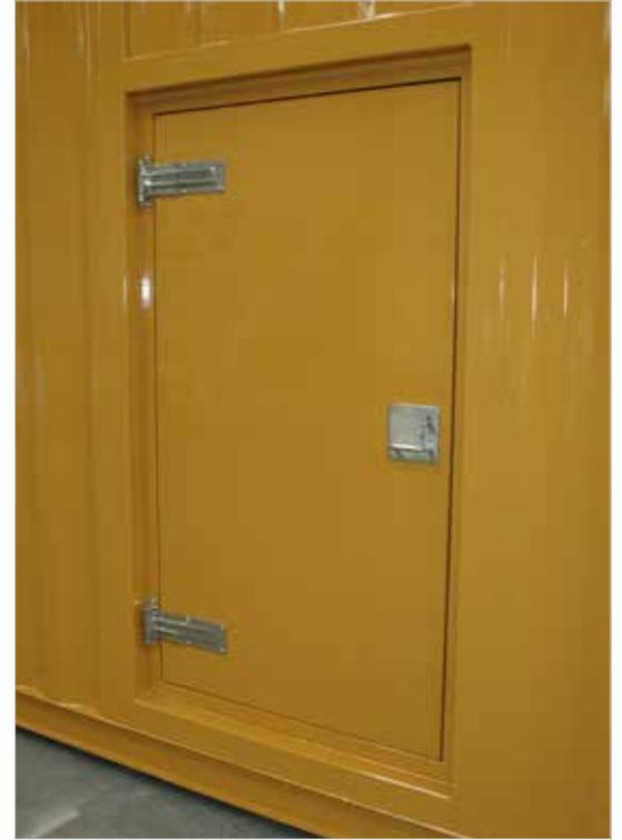
D100 Series Acoustic Doors are 100mm thick doors, made from durable sheet steel with an acoustic infill and a high quality compression seal for optimum noise reduction. They are suitable for high noise areas such as test or plant rooms and generator or machinery enclosures.
